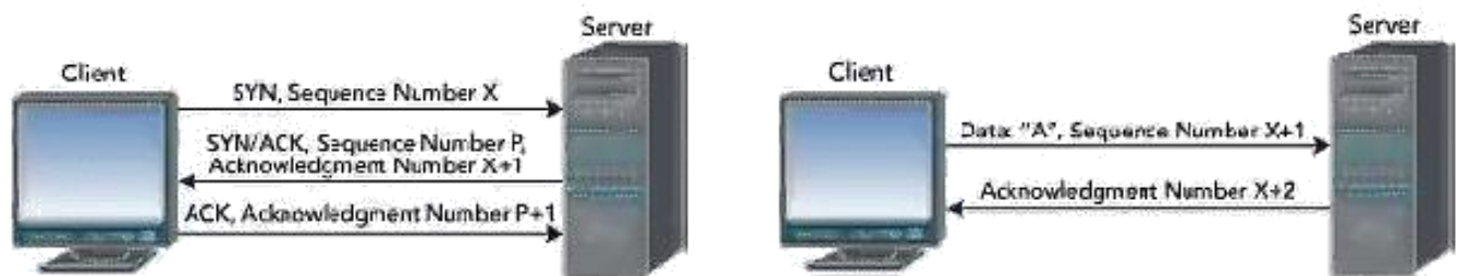
Fig: The three way handshake method for session establishment and sending Data over TCP
